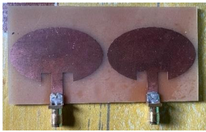
(a) Antena MIMO patch 2x2
